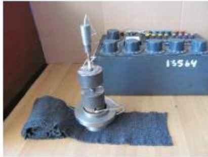
The unit for the measurement of round electrical conductivity of carbon fabric
